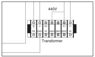
**Figure 5.** Rewiring the transform for 440V operation.
